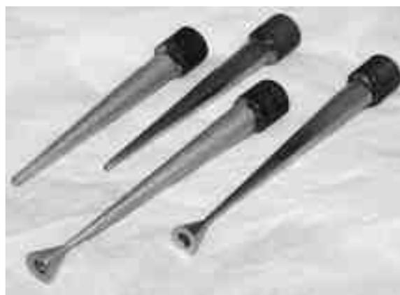
Fig. 8—Self-lubricating nanocrystalline nickel + molybdenum disulfide composite coating on hydraulic expansion mandrels.
