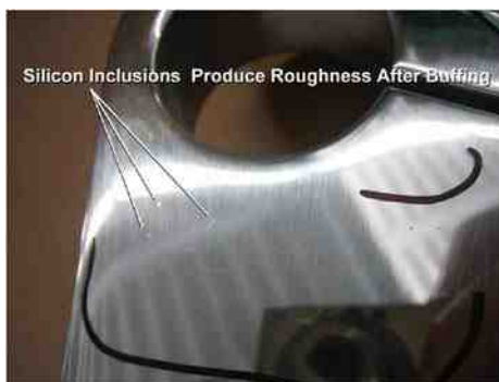
Figure 1—Effect of silicon inclusions on buffing.
