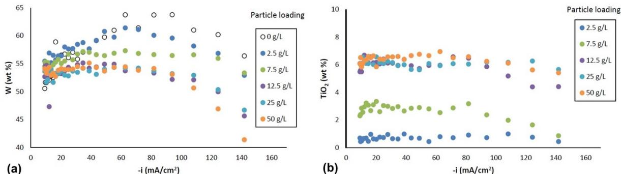
Figure 2 - Ni-W-TiO<sub>2</sub> deposit composition with variable particle loading: (a) wt% tungsten and (b) wt% TiO<sub>2</sub>.
