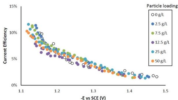
Figure 6 - Current efficiency with variable particle loading
