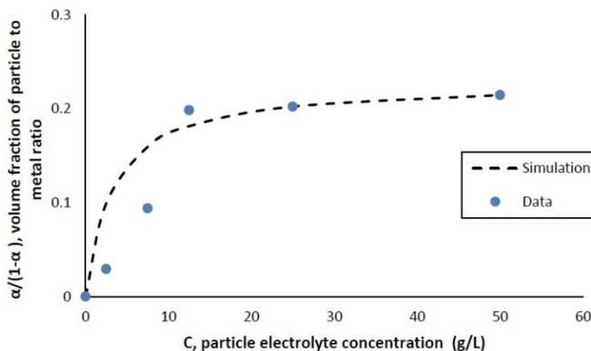
Figure 3 - Volume fraction ratio,  $\alpha/(1 - \alpha)$ , as a function of the particle electrolyte concentration comparing data with Gugliemi's model with fitted constants, cathodic current density =  $28 \text{ mA/cm}^2$  ( $-1.2 \text{ V}_{\text{SCE}}$ ).
