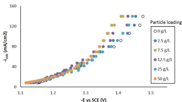
Figure 5 - Side reaction with variable particle loading.
