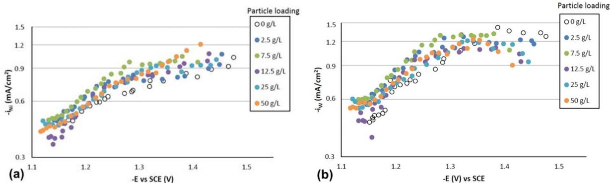
Figure 4 - Partial current densities with variable particle loading: (a) nickel and (b) tungsten.
