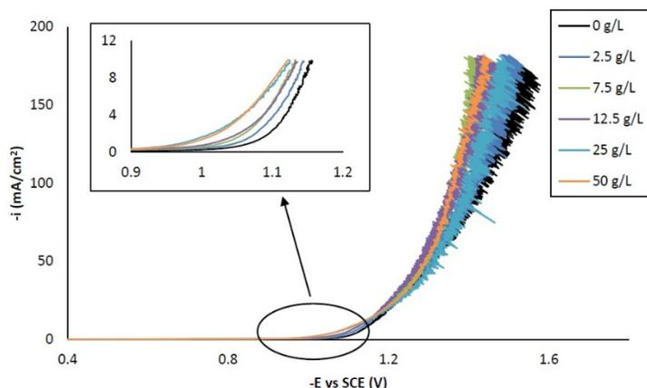
**Figure 1** - Polarization curves of the Ni-W-TiO<sub>2</sub> citrate-boric acid electrolyte at 500 rpm, 25°C, with 0, 2.5, 7.5, 12.5, 25 and 50 g/L titania microparticles.
