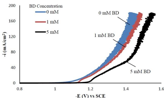
Figure 1 - Polarization curves of the Ni-W-TiO<sub>2</sub> citrate-boric acid electrolyte at 500 rpm, 25°C with 0, 1 and 5 mM BD.
