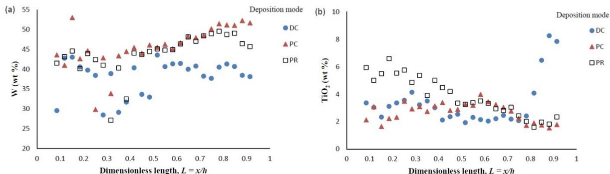
Figure 6 - Ni-W-TiO<sub>2</sub> deposit composition of (a) wt% tungsten and (b) wt% TiO<sub>2</sub> under DC, PC and PR conditions, in the presence of 5mM BD, with respect to a dimensionless length  $L$ , representing lower and higher current densities with smaller and larger values, respectively.
