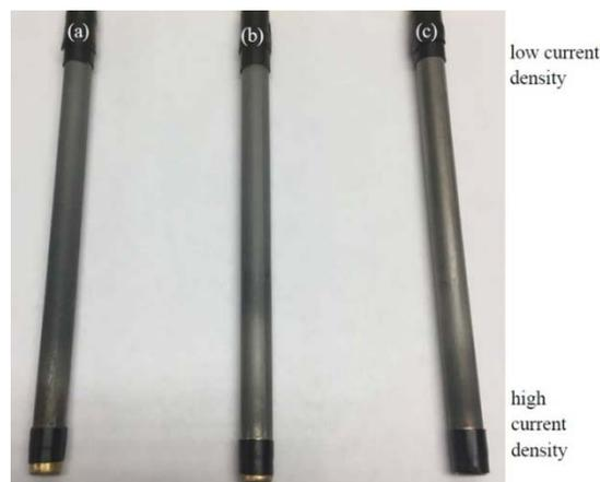
Figure 5 - Photographs of Ni-W-TiO<sub>2</sub> composite coatings plated with (a) 0 mM, (b) 1 mM and (c) 5 mM BD in the electrolyte for 30 min.
