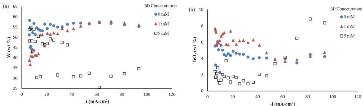
Figure 2 - Ni-W-TiO<sub>2</sub> deposit composition with variable BD concentration: (a) wt% tungsten and (b) wt% TiO<sub>2</sub>.
