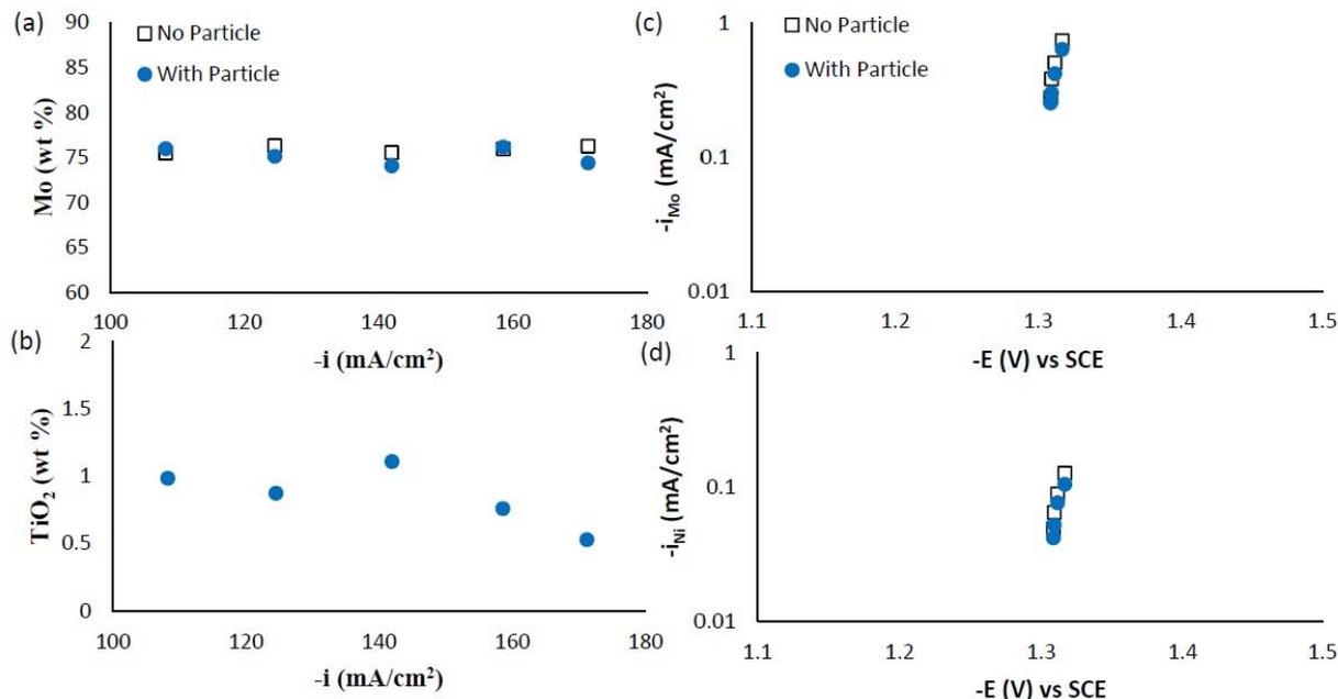
Figure 11 - Ni-Mo and Ni-Mo-TiO<sub>2</sub> deposit composition: (a) wt% Mo, (b) wt% TiO<sub>2</sub> and the partial current densities of (c) Mo and (d) Ni.
