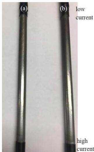
Figure 8 - Photographs of Ni-W-TiO<sub>2</sub> composite coatings plated with (a) PC and (b) PR, 5mM BD for a total time of 200 min (on-time: 120 min).
