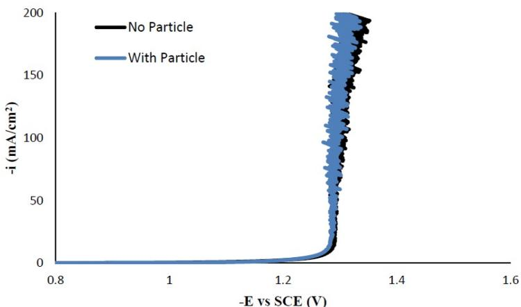
Figure 9 - Polarization curves of Ni-Mo deposition with and without TiO<sub>2</sub> particles.
