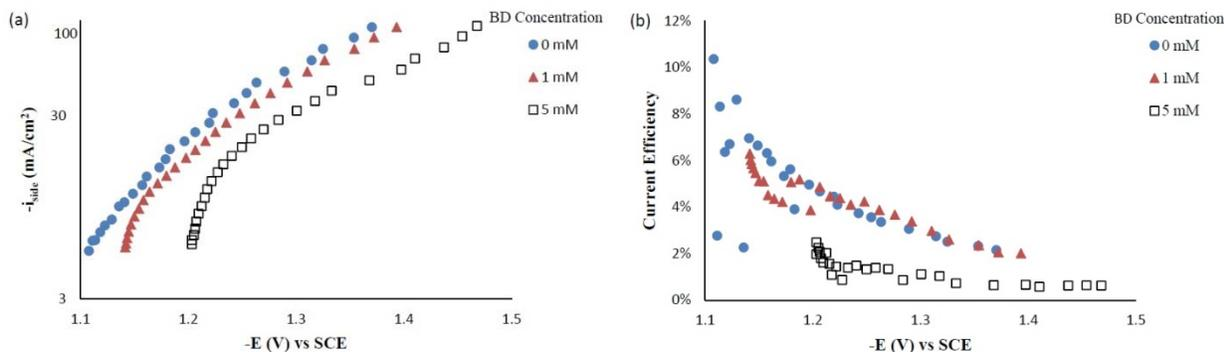
Figure 4 - Side reaction (a) and current efficiency (b) of Ni-W-TiO<sub>2</sub> composite deposition with variable BD concentration.
