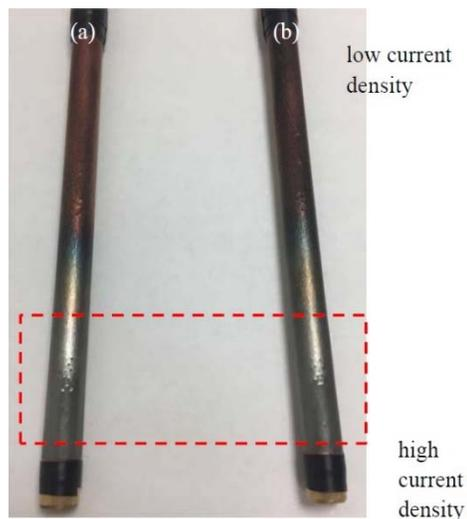
Figure 10 - Photographs of Ni-Mo coatings (a) without and (b) with the addition of 12.5 g/L titania particle loading in the electrolyte with 5mM BD.
