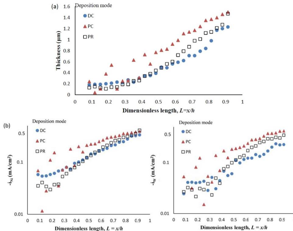
Figure 7 - Deposit thickness (a) and partial current density (b) of nickel and tungsten under DC, PC and PR conditions, in the presence of 5mM BD, with respect to a dimensionless length  $L$  representing lower and higher current densities with smaller and larger values, respectively.
