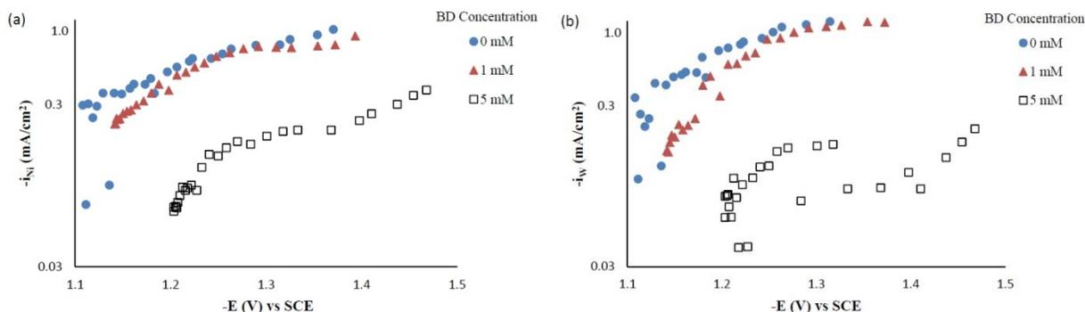
Figure 3 - Partial current densities of Ni-W-TiO<sub>2</sub> composite deposition with variable BD concentration: (a) nickel and (b) tungsten.
