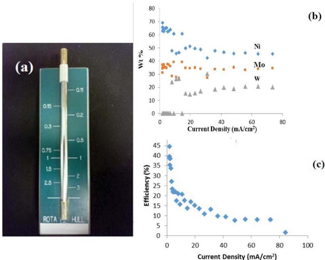
Figure 2 - Rotating Hull cell study of an electrolyte containing Ni, Mo and W at 500 rpm, at an average current density of 16.5 mA/cm<sup>2</sup>: (a) electrode and a scale representing a primary current distribution local current density estimate, (b) composition and (c) efficiency.
