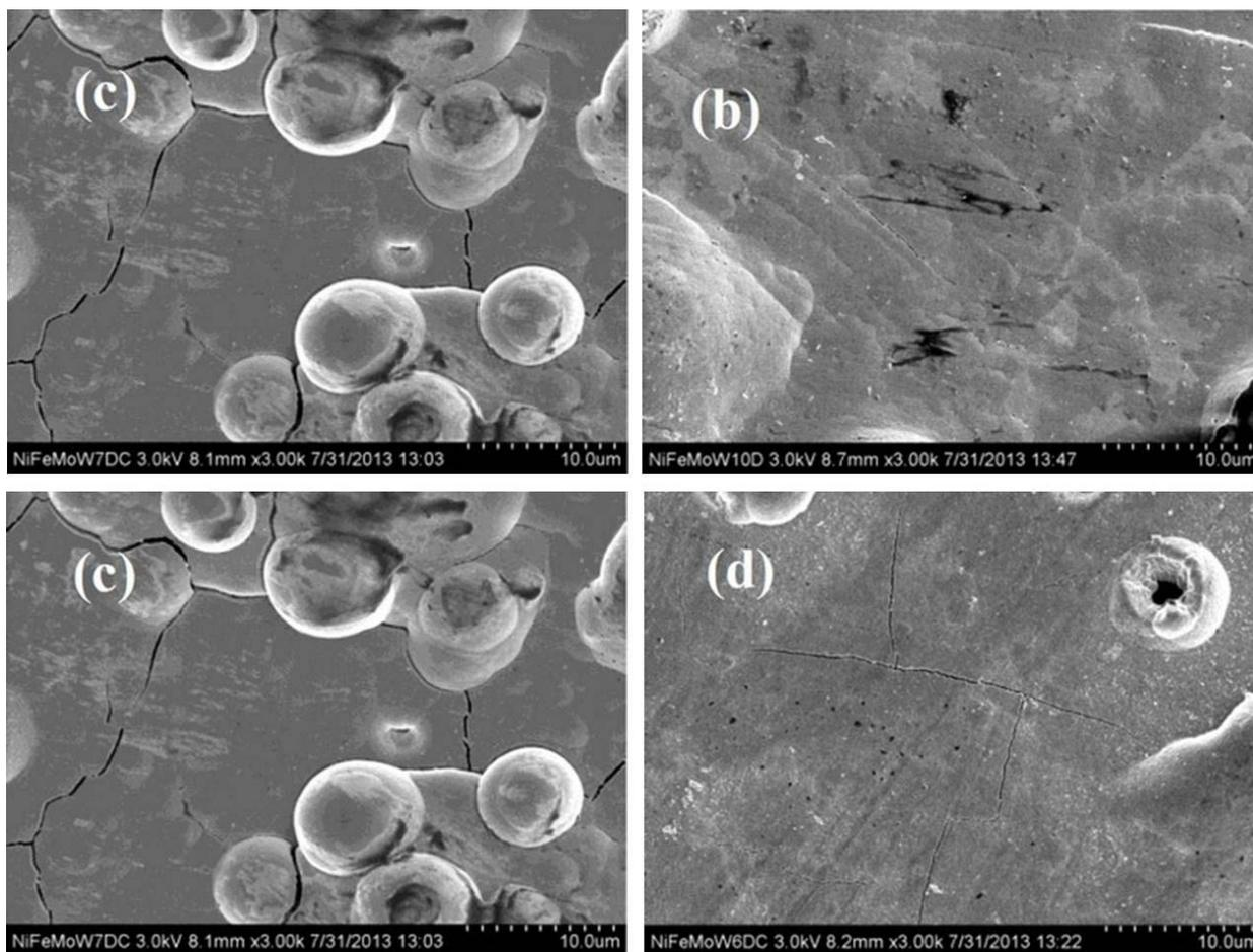
Figure 1 - SEM micrographs of the surface of deposits from an electrolyte containing Ni, Mo and W and variable amounts of Fe ions: (a) 0, (b) 0.05M, (c) 0.1M and (d) 0.15M, at 49.5 mA/cm<sup>2</sup>.
