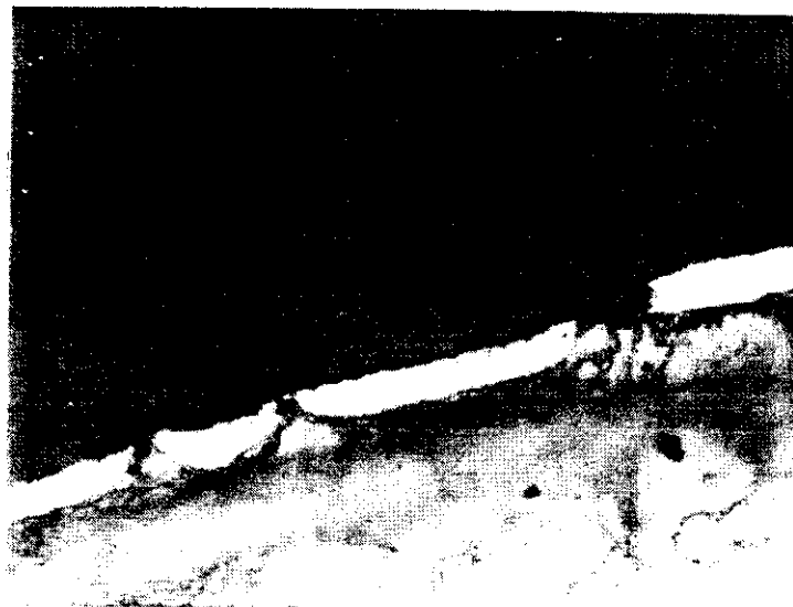
Cracked Nickel plate, 3 microns thick Cross Section, 1000 X
