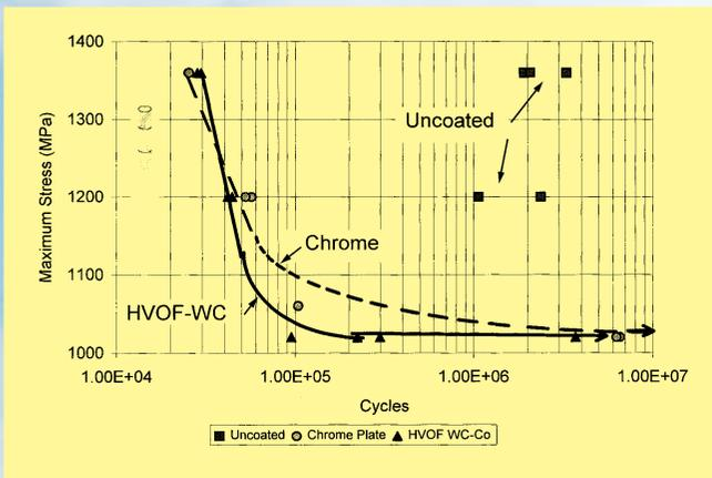
Fig. 4—Axial Fatigue Test Results:  $R = 0.1$ ,  $K_t = 1.035$  (Courtesy of Messier-Dowty<sup>7</sup>).
