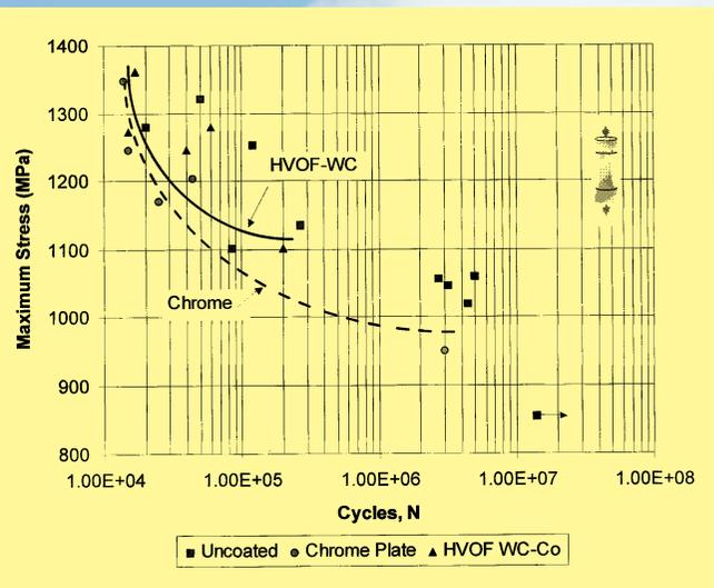
Fig. 5—Cyclic Fatigue Test Results—4340 Steel, Smooth Gage Specimens (adapted from Ref. 8).
