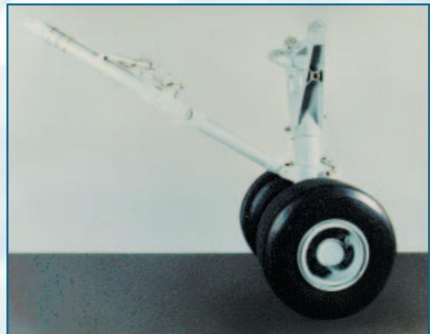
Fig. 1—Assembled landing gear.
