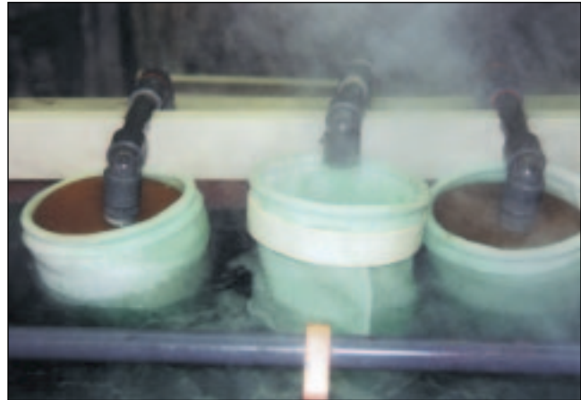
Filtration set-up on EN tank at Epner Technology to allow salt addition to working solution.
