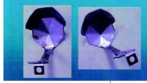
Steel Headlamp Reflector, Before & After Cleaning & Acid Pickling
