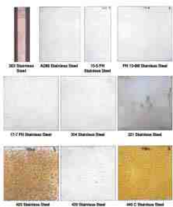
Fig. 6—Salt spray results for contaminated test specimens passivated in optimized citric acid.
