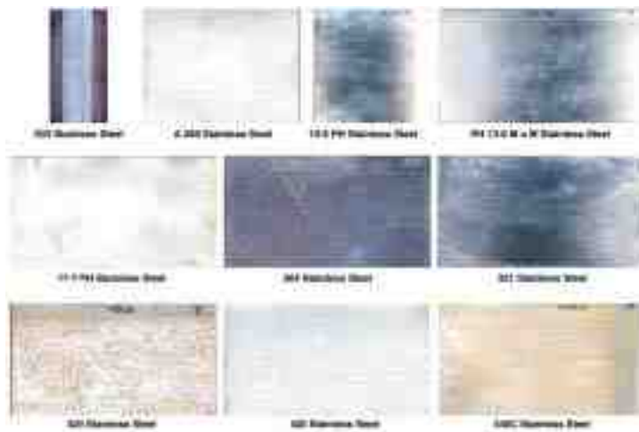
Fig. 1—As-received stainless steel test specimens subjected to two-hr salt spray. Test specimens did not receive a passivation treatment.
