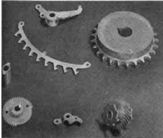
Figure 2—Steel parts plated in pyrophosphate copper bath for selective hardening.
