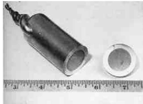
Figure 4—Part plated with 0.50-cm ( \frac{3}{16} -in.) thick copper in a pyrophosphate bath.
