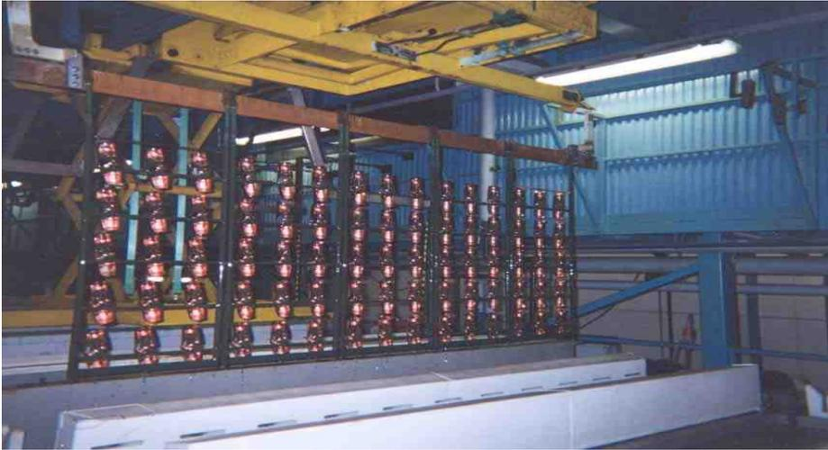
*Figure 8. Production parts through Direct Plate 3 process after acid copper plating*
