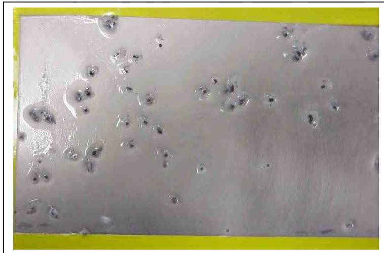
*Figure 11 A. Special EN 12  $\mu\text{m}$  on Mg.24 Hrs salt spray*
