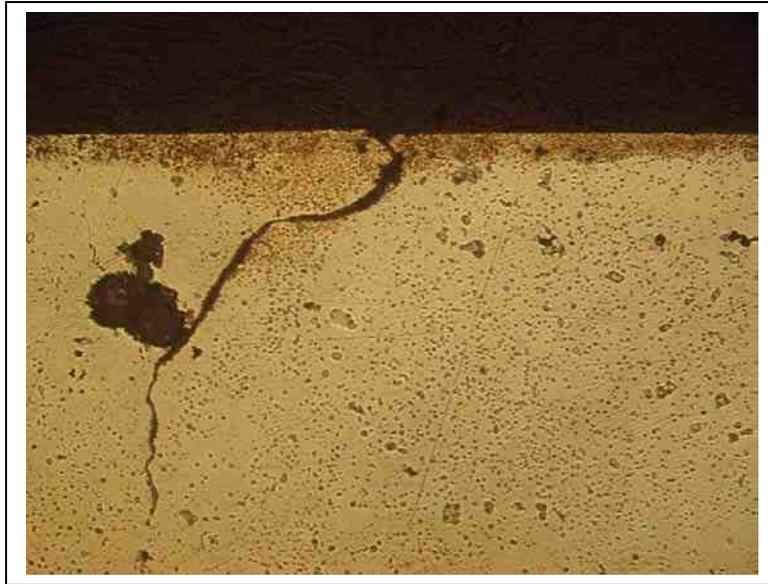
*Figure 10B. Cross-section of raw casting. 400X*
